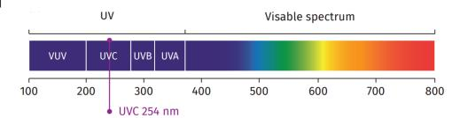
SCU-UV primary function is to neutralize pathogenic organisms and harmful chemical compounds in the supply air. The key principle is based on using ultraviolet germicidal irradiation (UGVI). UGVI is is electromagnetic radiation which inactivates microorganisms and its ability to reproduce by causing photochemical change in nucleic acids.
